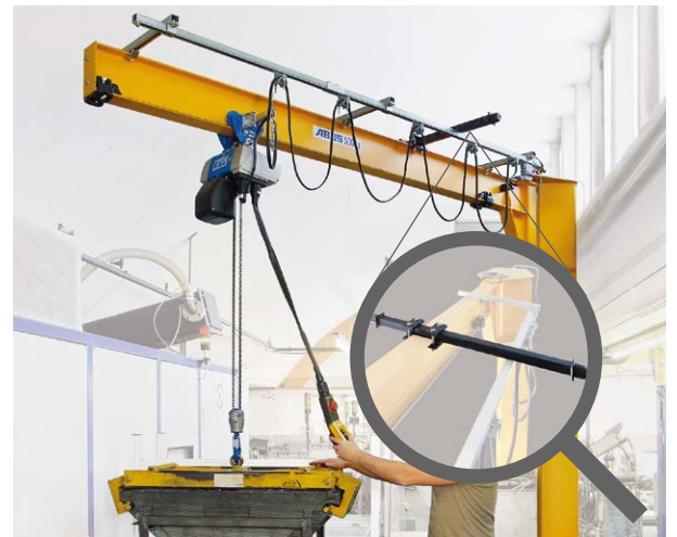
Slewing limit stop – bumper rod (Fig. 4)
