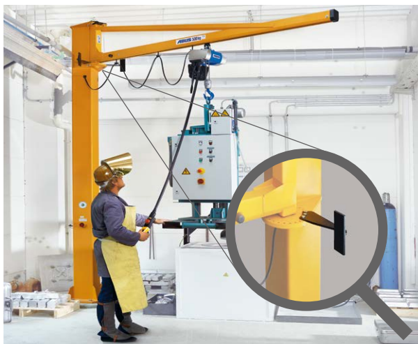
Slewing limit stops, adjustable (Fig. 5)
